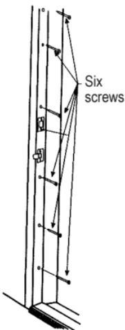
Drill pilot holes for the 2-1/2" wood screws for the lock side and run the screws in. You may need to work back and forth between the nailing and screwing, checking the margin between the frame and door.
