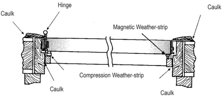
Install the hinge side compression type weather-strip in the same way you installed the lock side. Remember to first tack, make adjustments, and finish nailing.
