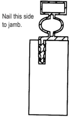
Now place a piece of paper or cardboard between the threshold and the jamb on the lock side.
