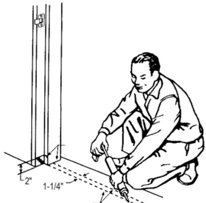
Apply caulk thoroughly to prevent water leakage
