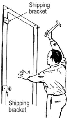
Tack two 6d nails in each corner to hold the door in place. Remove shipping brackets and plastic shipping protector. Check the door again for swing and centering.
