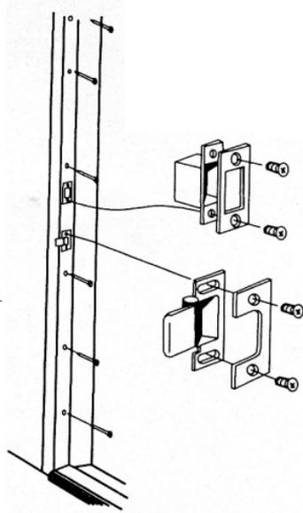
Next install the locks and dead bolt into the door. For installation instructions, refer to the manufacturer's instructions that come with them. Adjust the strike plate for proper fit.
