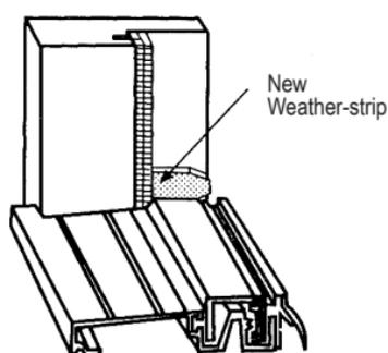
Peel the paper backing off and place these on the bottom of the jamb against the threshold as shown.
